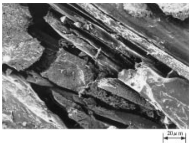
Fig. 17. Magnified SEM photograph of fracture surface.
