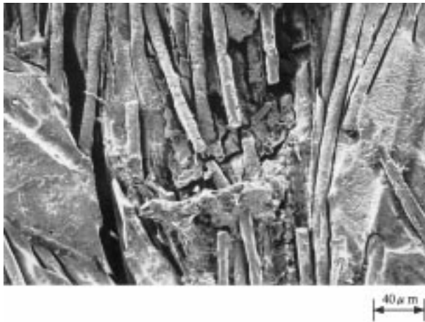
Fig. 15. SEM photograph of fracture surface.
