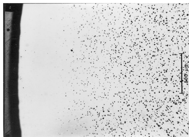
Fig. 5. Typical feature of the Yb added sample with a thin circumferential dense layer followed by an increasing amount of porosity towards the core of the sample.
