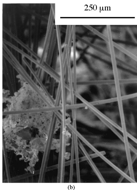
Fig. 18. SEM micrograph of the surface of filter A (a) and filter B (b) in contact with the cerium oxide deposit after calcination at 1100°C.
