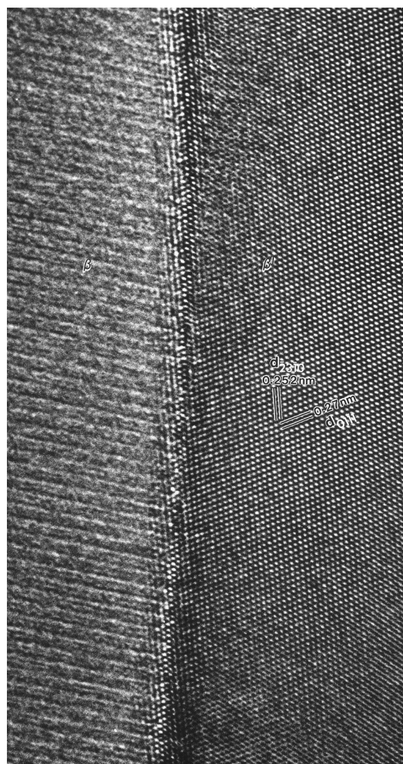
Fig. 6. HREM micrograph showing the interface between \beta -sialon and \beta - \text{Si}_3\text{N}_4 grains. The \beta -sialon grain is oriented along the [4\bar{1}56] zone axis. The absence of any intergranular glassy phase may be noticed.
