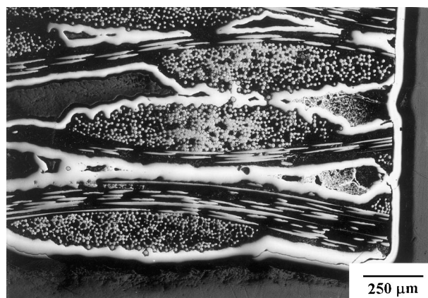
Fig. 1. Cross-section of SiC/SiC composite, showing fiber bundles.
