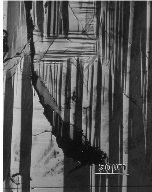
Fig. 3. Surface relief showing close relation with band structures.
