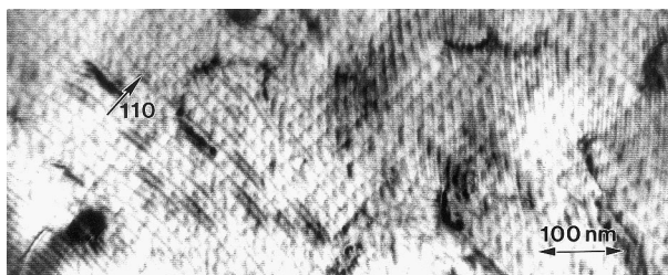
Fig. 8. Plan-view TEM image of a \text{Mg}_2\text{SnO}_4 film grown by solid–solid reaction on a \text{MgO} substrate. The arrow indicates a \langle 110 \rangle direction.
