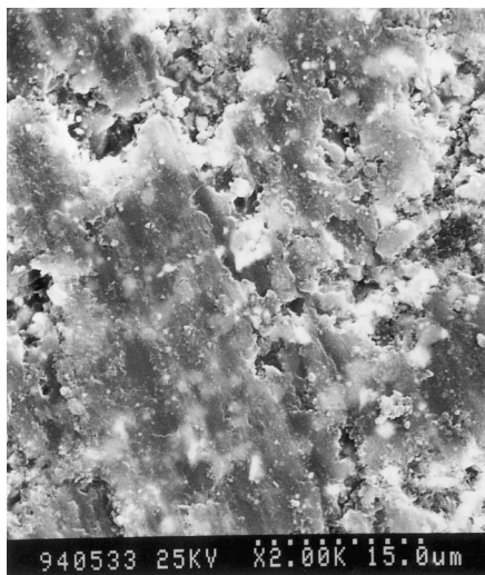
Fig. 7. SEM micrograph of the worn surface of ABW05 specimen sliding in air at 800°C.
