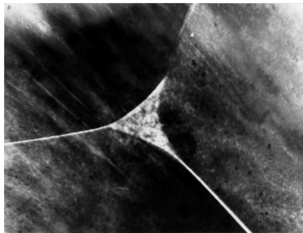
Fig. 1. Grain boundary triple junction of PMN–PFN solid solution sample (magnification 50×).
