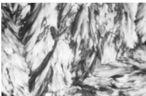
Fig. 6. Photomicrograph of M20 (850°C, 3 h + 1000°C, 10 h). Coarse feathery crystals of diopside surrounded interlocked euhedral to subhedral of anorthite and forsterite C.N.×360.
