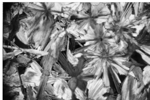
Fig. 8. Photomicrograph of M40 (850°C, 3 h + 1000°C, 10 h). Part of the section exhibits crosshatching twinning of microcline intergrowths with long fibrous of diopside C.N.×360.
