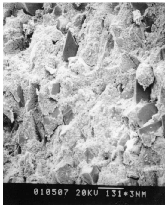
Fig. 10. SEM micrograph of fracture surface of the gelcast RSiC green bodies.
