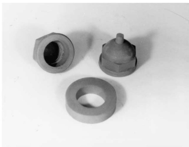
Fig. 8. Complicated shapes of SiC green bodies prepared by gelcasting.
