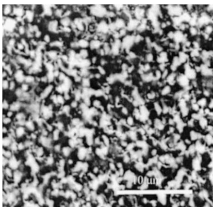
Fig. 5. Typical microstructures of the polished surface of B_4C/40 wt.% (W,Ti)C composite.
