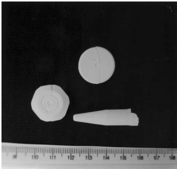
Fig. 8. Gelcast and air-dried preconsolidated \text{Al}_2\text{O}_3 part geometries.
