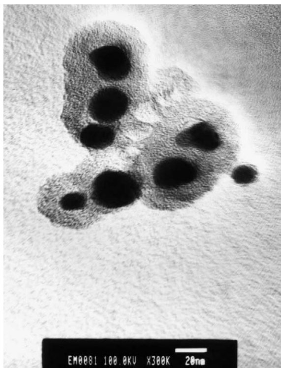
Fig. 3. Detailed TEM image of iron particles encapsulated in the carbon nanocapsules.
