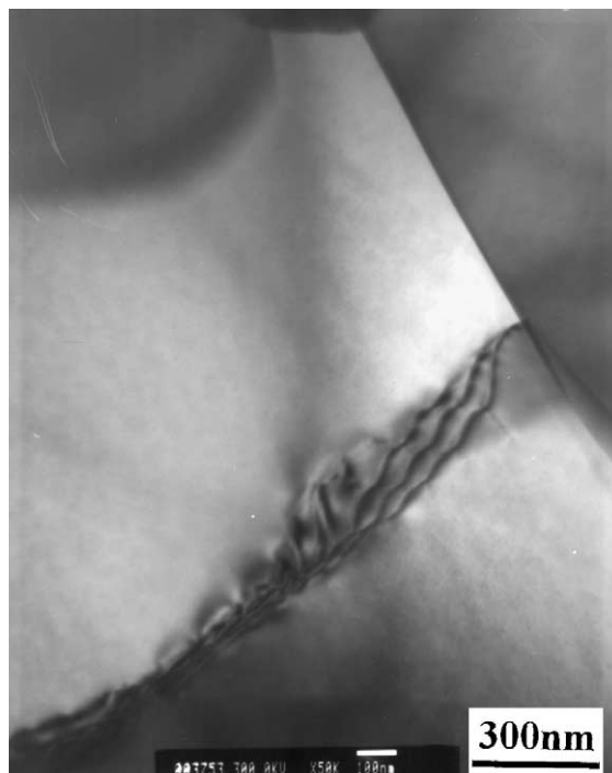
Fig. 9. TEM micrograph of as sintered 10 vol.% \text{Cr}_3\text{C}_2/\text{Al}_2\text{O}_3 composite showing dislocations pile-up at subgrain.
