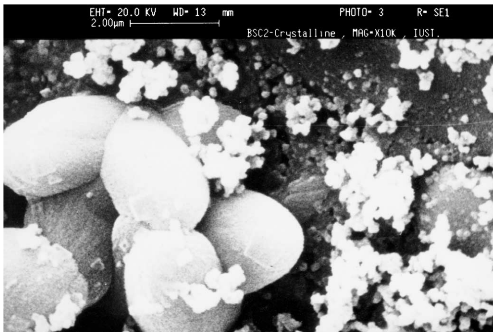
Fig. 6. SEM micrograph of glass specimen BSC1 after crystallisation at 723 °C for 1 h.
