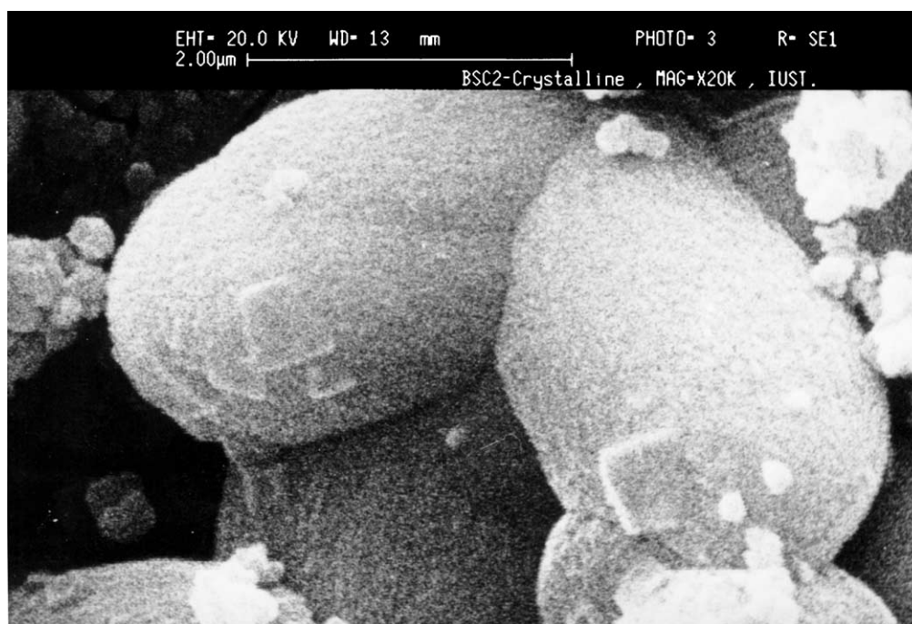
Fig. 8. Enlarged SEM micrograph of specimen BSC1 after crystallisation at 723 °C for 1 h, showing BaB 2 O 4 ellipsoids.
