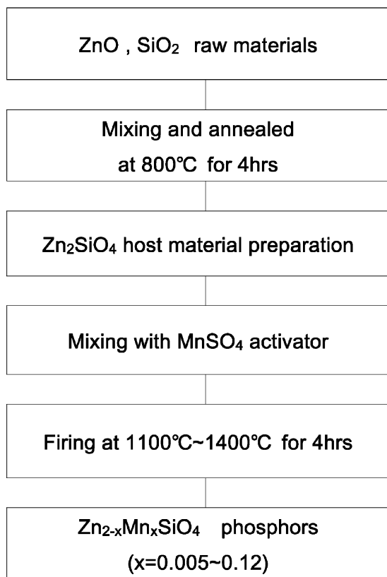
Fig. 1. Flow chart for the sample preparation of \text{Zn}_{2-x}\text{Mn}_x\text{SiO}_4 phosphors prepared with the solid-state reaction method.
