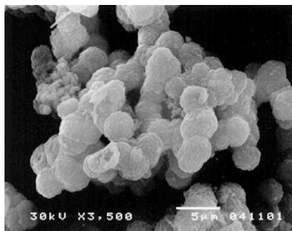
Fig. 5. Scanning electron micrograph of powders obtained by the reaction of zirconium tetra n -propoxide in 1,4-butanediol (ZNP concentration of 0.4 mol/dm 3 ) and cooling autoclave once the temperature reached 250 °C.
