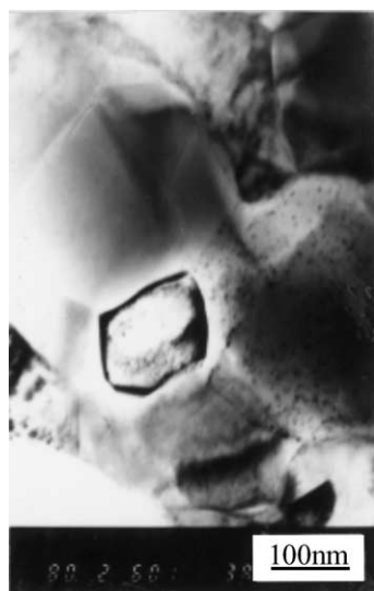
Fig. 2. TEM micrograph showing the location of nano TiN particles.
