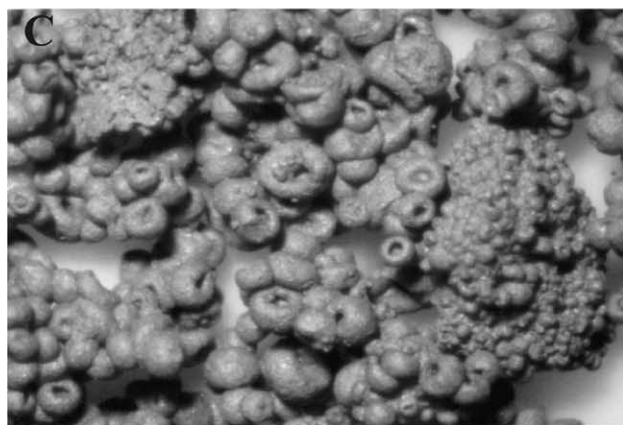
Fig. 4. Morphological aspects of ZA-4 clay grains: (A) detail of the inner part of a grain; (B) several individual grains; (C) formation of agglomerates from small grains.
