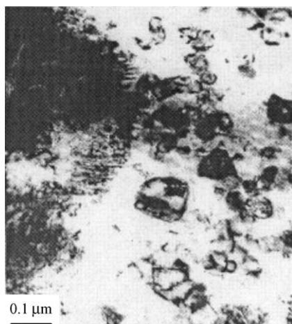
Fig. 6. TEM photograph of distortion induced Martensite in the interface.
