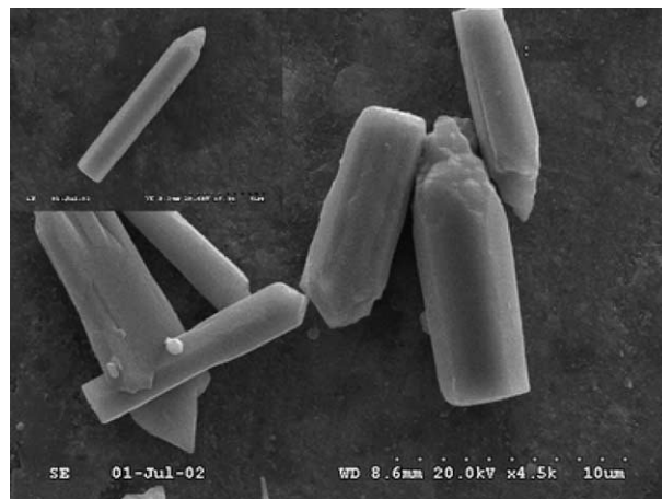
Fig. 2. SEM ZnO powder hydrothermally prepared at 200 °C for 2 h.
