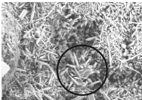
Fig. 5. Aluminium borides in formation. Sintering at 1373 K, 30 min.
