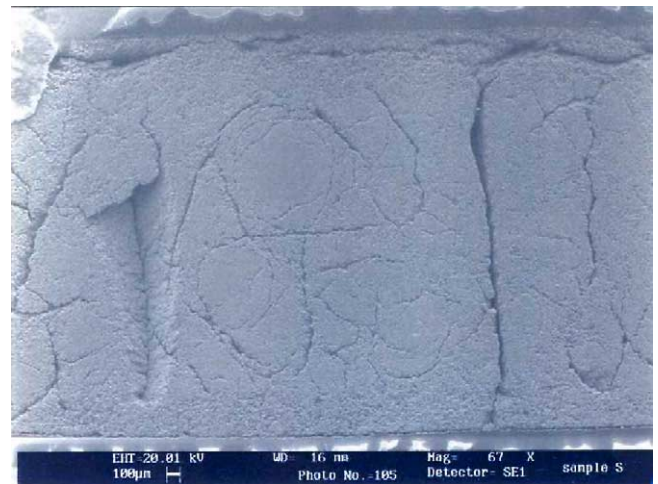
Fig. 7. SEM micrograph of polished section of the sample A oxidized at 1100 °C for 96 h.
