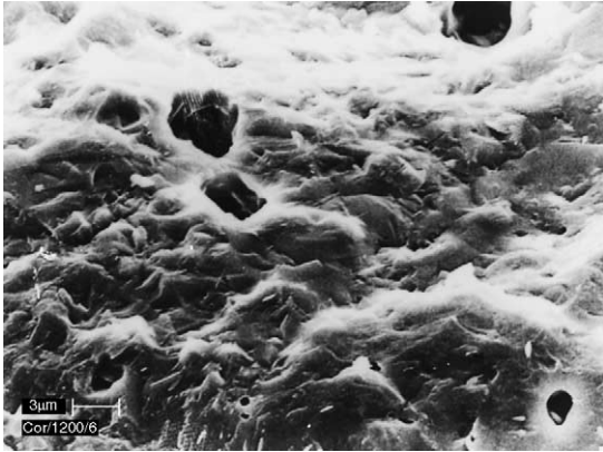
Fig. 6. SEM photomicrograph of sample fired at 1200 °C for 6 h.
