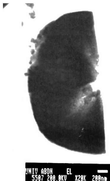
Fig. 3. Transmission electron micrograph of one of the smaller spheres in Fig. 2, showing hollow core and fibrous, radiating structure.
