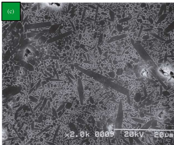
Fig. 9. SEM micrographs of the specimens gas-pressure sintered at 1850 °C for 3 h: (a) 2 μm, (b) 7 μm and (c) 25 μm.
