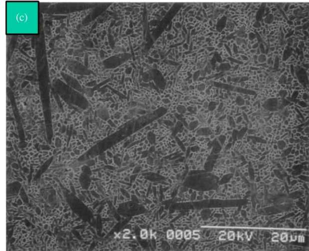
Fig. 10. SEM micrographs of the specimens gas-pressure sintered at 1900 °C for 3 h: (a) 2 μm, (b) 7 μm and (c) 25 μm.
