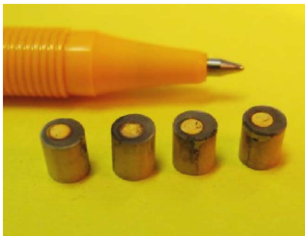
Fig. 6. Samples for electromechanical characterisations and integrated transducers [8].
