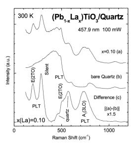
Fig. 3. Raman spectra (300 K) under excitation of 4579 Å and 100 mW, from (a) x = 0.10 (Pb<sub>1-x</sub>La<sub>x</sub>)TiO<sub>3</sub> quartz, (b) bare quartz region, and (c) difference of (a-b).
