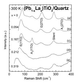
Fig. 1. Raman spectra taken at 300 K under excitation of 457.9 nm and 100 mW, showing the major PLT phonon bands below  $400\,\mathrm{cm}^{-1}$ , from MOCVD-grown (Pb<sub>1-x</sub>La<sub>x</sub>)TiO<sub>3</sub>/quartz for *x* values of: (a) 0, (b) 0.054, (c) 0.167, (d) 0.212, and (e) 319.
