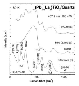
Fig. 4. Raman spectra (80 K) under excitation of 4579 Å and 100 mW, from (a) x = 0.10 (Pb<sub>1-x</sub>La<sub>x</sub>)TiO quartz, (b) bare quartz region, and (c) difference of (a-b).
