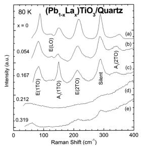
Fig. 2. Raman spectra taken at  $80\,\mathrm{K}$  under excitation of  $457.9\,\mathrm{nm}$  and  $100\,\mathrm{mW}$ , showing the major PLT phonon bands below  $400\,\mathrm{cm}^{-1}$ , from  $(\mathrm{Pb}_{1-x}\mathrm{La}_x)\mathrm{TiO}_3/\mathrm{quartz}$  for x values of: (a) 0, (b) 0.054, (c) 0.167, (d) 0.212, and (e) 0.319.
