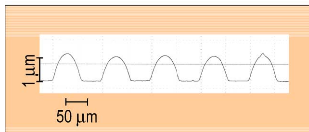
Fig. 1. Optical photograph of \text{SnO}_2 micropattern formed on the hydrophobic–hydrophilic patterned surface using the precursor solution from \text{SnCl}_2 , and the surface profile of the micropattern.
