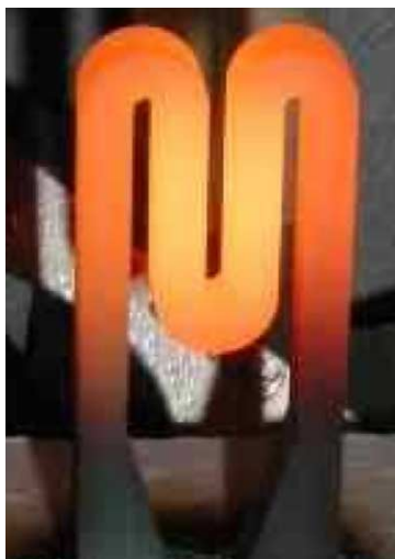
Fig. 6. Heating element of 211 glowing at 1350 °C.
