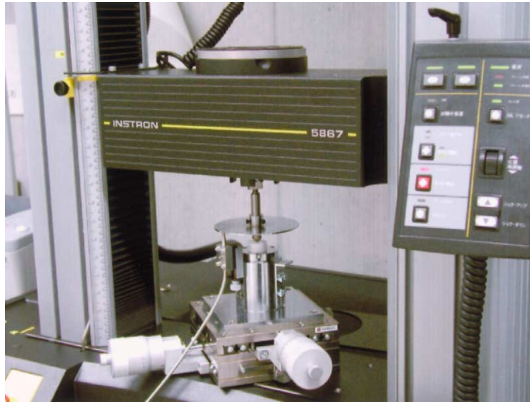
Fig. 1. An overall view of quasi-static indentation testing system.
