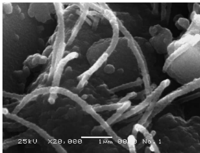
Fig. 3. Micrograph of the \text{Al}_2\text{O}_3 –5% \text{MgB}_2 composites sintered at 850^\circ\text{C} .
