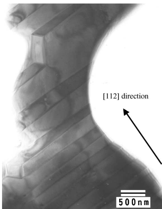
Fig. 3. Low magnification TEM image from [1 -1 0] zone.
