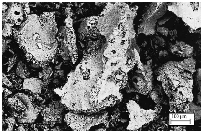
Fig. 6. SEM photograph of the ash obtained at LSM ions: sucrose mole ratio 1:2.
