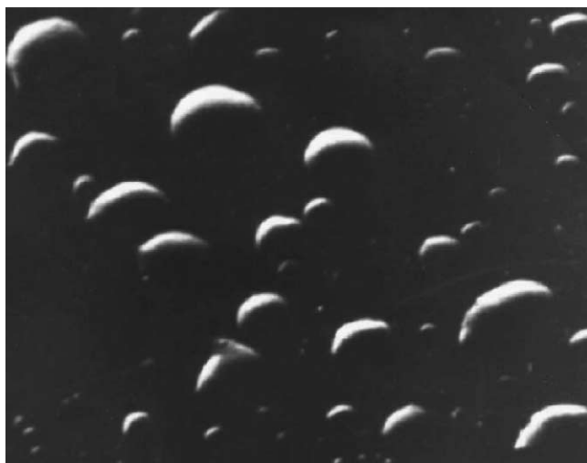
Fig. 7. SEM of B 1 glass heat-treated at 550 °C for 30 h (350 \times ).
