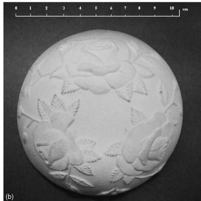
Fig. 4. The surface structure of the molds used in the SS casting using: (a) ES and (b) ES/ATB binder systems (sintered at 1600 °C for 2 h).
