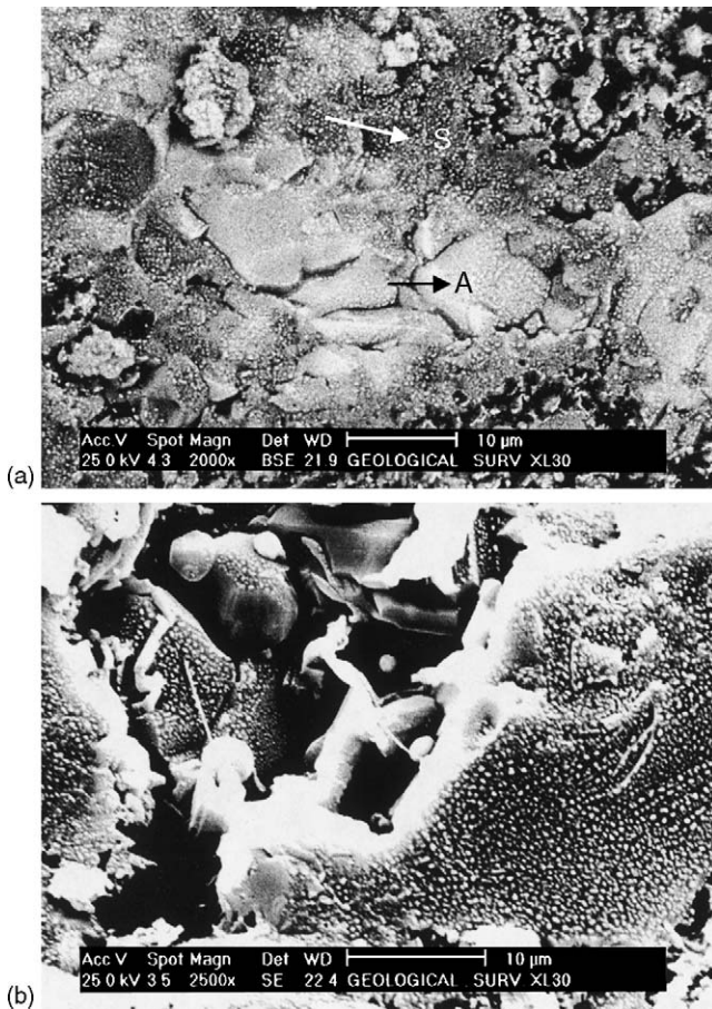
Fig. 8. SEM photomicrographs and EDS analysis of sintered M3 composite.
