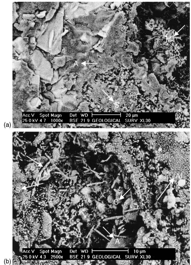
Fig. 10. SEM photomicrographs of sintered M4 composite.
