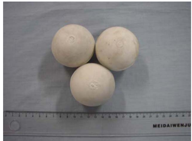
Fig. 8. Sintered alumina balls (the linear shrinkage rate was 16.4% after sintering and the final diameter was 5.6 cm).
