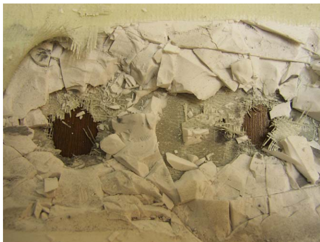
Fig. 5. Fracture image of the AM2 ceramic (view of a backface of the plate) after ballistic impact with 7.62 \times 51 -mm NATO Ball FMJ (backing material was taken out).
