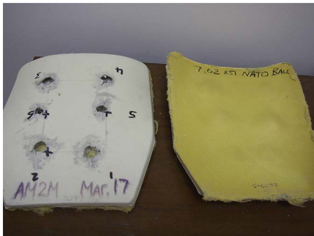
Fig. 4. Ballistic test result of the armour plate ( 7.62 \times 51 -mm NATO Ball FMJ). Left: front view and right: back view.
