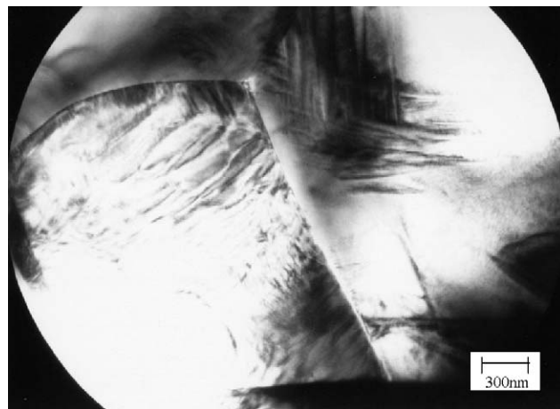
Fig. 2. STEM observation of ceramic H–Ni.
