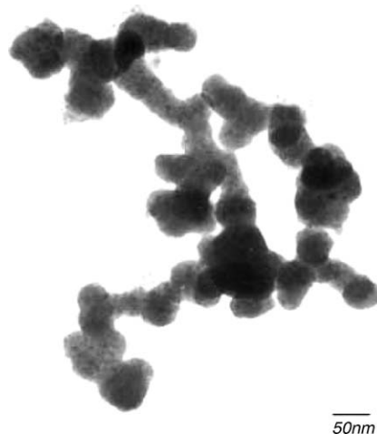
Fig. 5. TEM micrograph of KLN powder obtained at 900 °C (pH 8).
