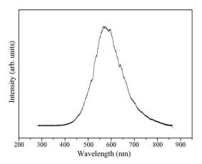
Fig. 4. Room temperature PL spectrum of the products with an excitation wavelength at  $325\ \mathrm{nm}$ .
