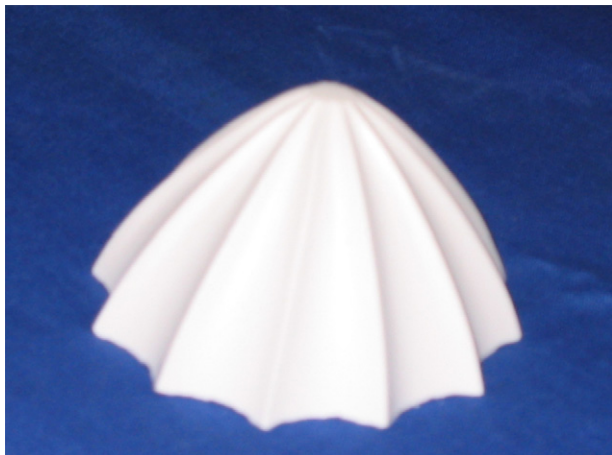
Fig. 9. Green body obtained by gel-casting technology without de-airing step.
