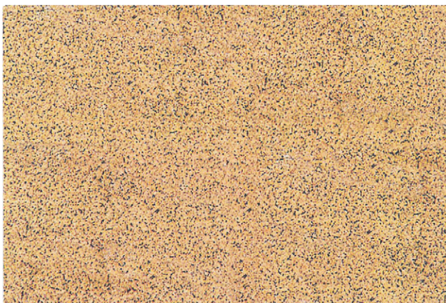
Fig. 10. Glass G1.5 Z heat-treated at (680 °C, 1 h + 1050 °C, 1 h). Almost similar to above but of finer texture P.N., \times 400 .
