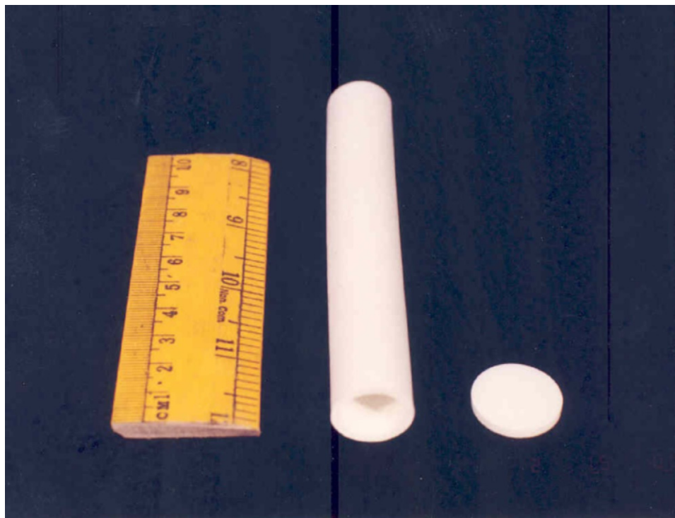
Fig. 9. Photograph of alumina membrane substrate in tubular and planar configuration prepared by gelcasting (sintered at 1350 °C, porosity 71.6%).
