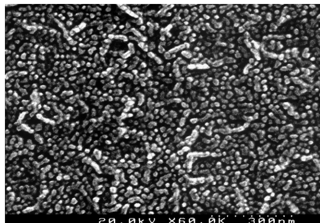
Fig. 7. SEM micrograph of the Al-(ZnO/PAN) 20 film.
