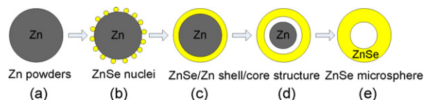
Fig. 7. Schematic illustration of growth mechanism of ZnSe microspheres prepared by hydrothermal synthesis.
