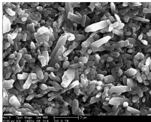
Fig. 3. SEM morphology of as-etched Nd- \alpha -sialon ceramics.
