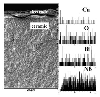
Fig. 6. EDS analysis of  $(Bi_{1-x}Cu_x)(Nb_{1-x}W_x)O_4$  ceramics.
