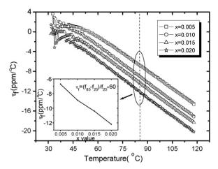
Fig. 5. The temperature coefficients of resonant frequency of  $(Bi_{1-x}-Cu_x)(Nb_{1-x}W_x)O_4$  ceramics.
