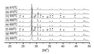
Fig. 2. XRD patterns of  $(Bi_{1-x}Cu_x)(Nb_{1-x}W_x)O_4$  ceramics for x = 0.005 (a), x = 0.010 (b), x = 0.015 (c–e) and x = 0.020 (f–h) at different sintering temperature (\*:  $\alpha$ -phase; o:  $\beta$ -phase).
