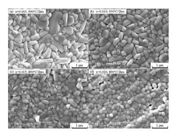
Fig. 3. SEM micrographs of  $(Bi_{1-x}Cu_x)(Nb_{1-x}W_x)O_4$  ceramics.
