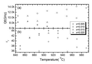
Fig. 4. Microwave dielectric properties as a function of sintering temperature for  $(Bi_{1-x}Cu_x)(Nb_{1-x}W_x)O_4$  ceramics.
