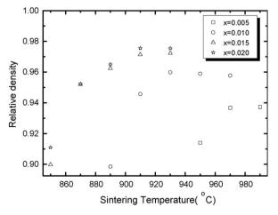
Fig. 1. The density of  $(Bi_{1-x}Cu_x)(Nb_{1-x}W_x)O_4$  ceramics as a function of sintering temperature.
